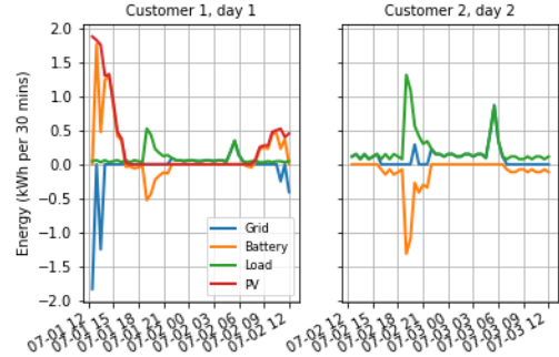
Fig. 4. Energy flows for two customers during the battery exchange.
